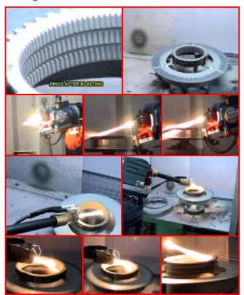
MEC is specialized in developing customized Automatic Thermal Spray System, which are targeted to fulfill the customer specific requirements.
