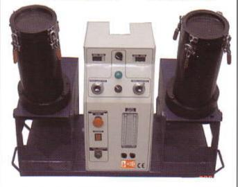
Designed for non-stop continuous operation for same or different powders. Both canisters are of 3350 cc capacity.
