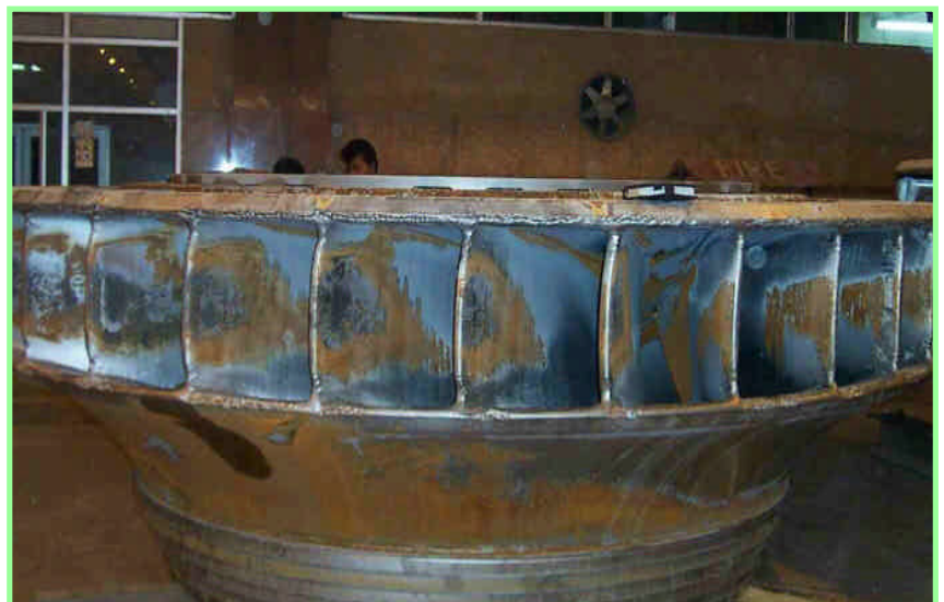
Fig 2 : Un-coated Hydro Turbine Component (Runner)
