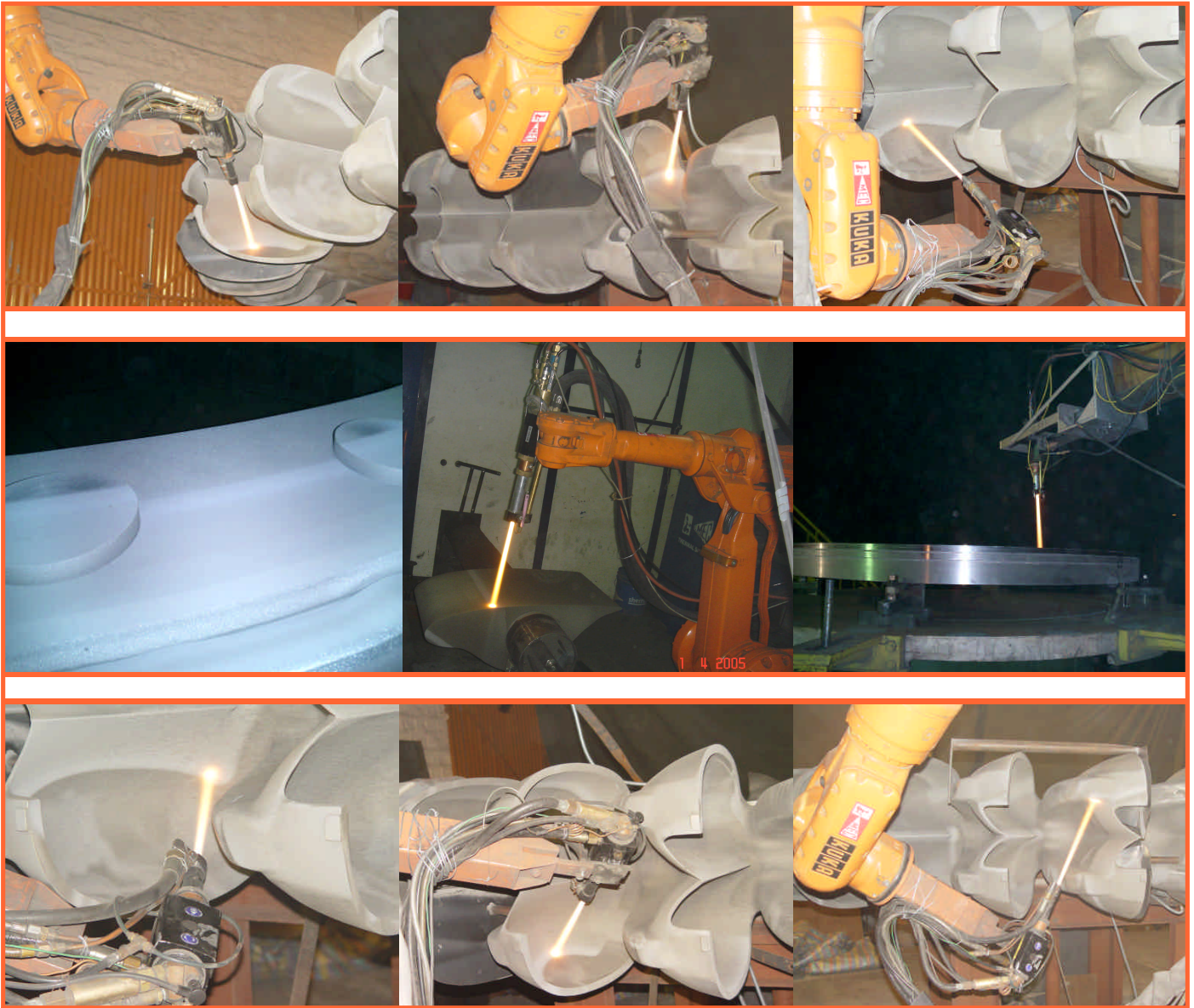
Fig 1 : Coating of Guide Vane and Pelton Wheel using HVOF System & allied by Robotics for efficient coating processes.
