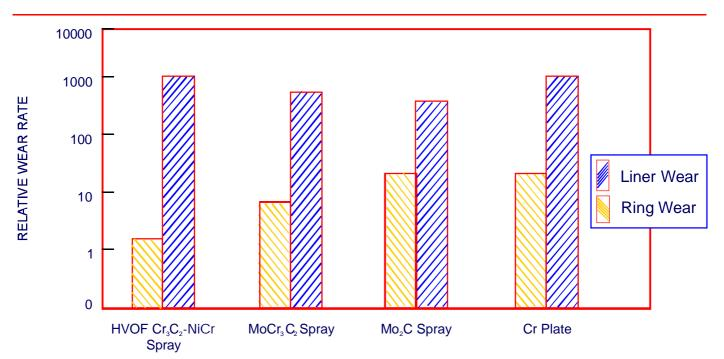
Fig. 3 : Summary of the piston ring coating and cylinder liner wear results under steady state condition engine tests comparing thermally sprayed coatings and electroplated chromium
