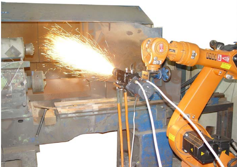
ARCJET 96- ED spray gun mounted on KUKA robot for automated operation
